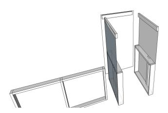
Add the walls to the tower. Use the pieces that don't have a recessed end (it's a little easier in that either end works). Screw from the wall into the tower, into the support on the inside.
